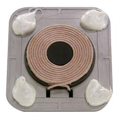
Figure D-2: 100% Silicone applied to transmitter
